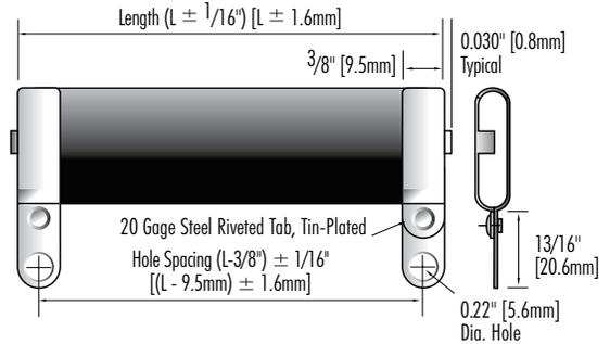
**Figure 3. With Right Angle Radial Tabs - same direction - (G2)**
