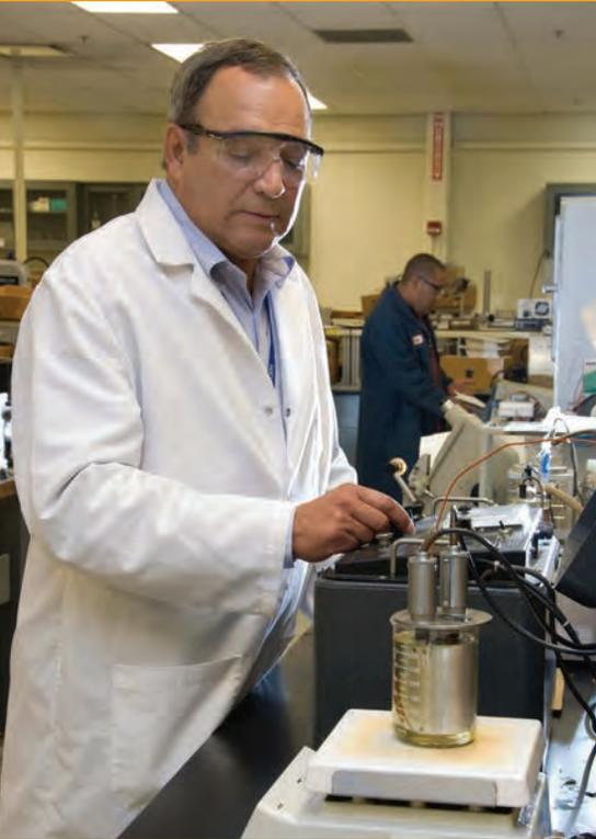
Aerovox capacitors undergo 100% electrical testing including: Accelerated Life Testing (ALT) for 2000 hours at 125% voltage rating and temperature at 10°C greater than maximum rating, fault current, and mechanical testing. The SuperMet line is designed to meet performance testing outlined in the Electrical Industry Association (EIA) standard #RS-456A.
