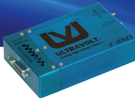
The E Series of precision high-voltage power supplies has very low ripple, excellent linearity, and very stable temperature characteristics. Models in this series are offered with a 10ppm temperature coefficient and reference. The control and monitoring functions are available on a standard DB15 female connector.
