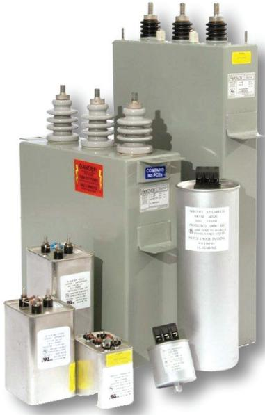
Aerovox manufactures both single-phase and three-phase power factor correction capacitors up to 4,800 VAC. Our AeroPower brand PFC capacitors are designed for high reliability applications, and have a life rating of over 200,000 hours. They are designed to withstand harmonic currents, with special high harmonic versions available.
