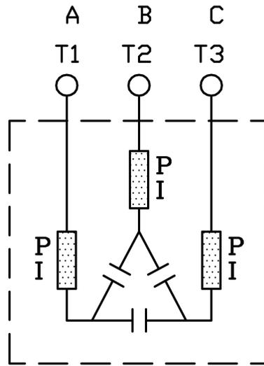
Internal Schematics for Low Voltage
