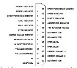
All logical indicators are open collector outputs rated at 16V (max) in the off state. An internal  $100\Omega$  resistor is connected in series with the open collector transistor. The pull down voltage is 0.9V plus the internal resistor drop.
