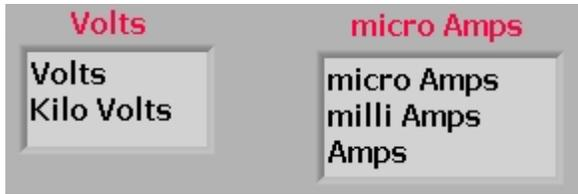
When the Channel B is changed from Volts to Kilo Volts, and Channel C is changed from micro Amps to milli Amps, the ‘Set points and Monitors’ tab will display the data as shown below.
