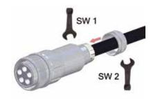
Screw cable gland cap (2) to cable gland basis (4)
