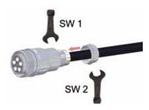
Screw cable gland cap to cable gland basis
