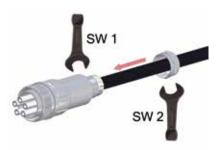
Screw cable gland cap (3) to cable gland basis (4)
