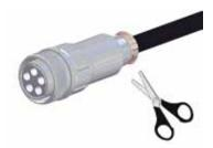
Cut overlapping shield braid ⚠ Carefully remove shield strands. Loose strands can cause electrical break down
