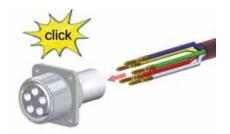
Slide contacts completely into connector shell until contacts snap into place
