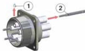
Remove snap rings (1) and take out male contacts (2)
