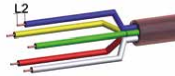
Remove dielectric insulation of single wires (L2 = 5mm) ⚠ Do not damage conductors
