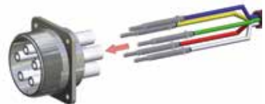
Slide single wires completely into insulation tubes
