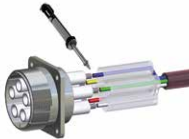
Solder one conductor on each female contact
