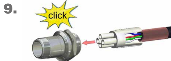
Put insulation part (2) into housing (3) 🗨 Pay attention to notches.
