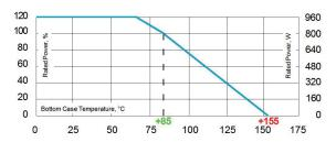
Derating (thermal resist.) UXP-800: 9.09 W/K (0.11 K/W) Power rating: 800 W at 85°C bottom case temperature\* Please ask for detailed mounting procedure!
