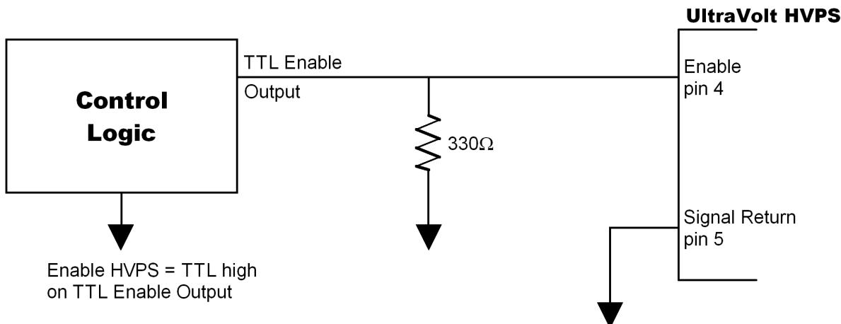
The 330Ω resistor will ensure that with a low TTL Enable Output signal, the required 1mA will be drawn from the UltraVolt HVPS *Enable/Disable* terminal, thus forcing the HVPS to be in the disabled state. When the TTL Enable Output signal goes high, the high-voltage power supply is prevented from sinking the required current and, therefore, the HVPS is in the enabled state.
