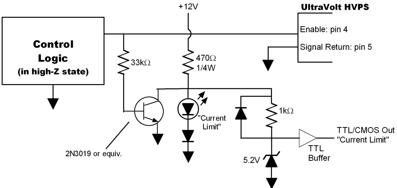
The above circuit is a slight modification of the one in part a), operating in the same way, except when the L.E.D. is lit the TTL buffer is enabled. The 5.2V Zener diode serves to prevent any harmful transients from reaching the TTL buffer (or any other TTL logic gate). This circuit is ideal for automated systems.
