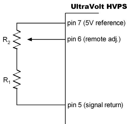
$$\begin{aligned} &\text{output} \\ &\left(\frac{R_2}{R_1 + R_2 + 464\Omega}\right)(V_{\text{out max}}) \\ &\text{to} \\ &\left(\frac{R_1 + R_2}{R_1 + R_2 + 464\Omega}\right)(V_{\text{out max}}). \end{aligned}$$
