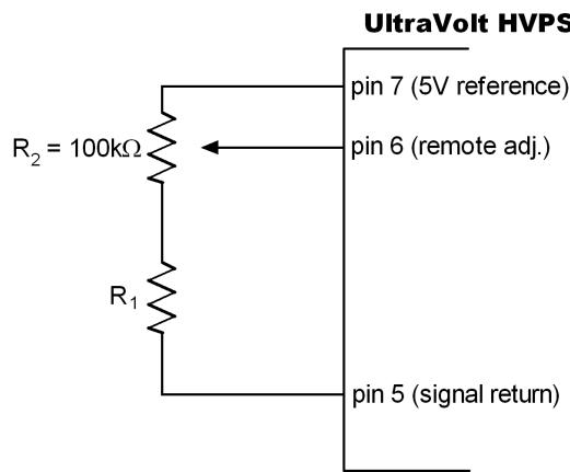
With output up to  $-1500\text{V}$  and  $R_2 = 100\text{k}\Omega$ , find  $R_1$  for a  $-E_0$  unit.  $V_{\text{out}}$  for supply rated 2000 volts,
