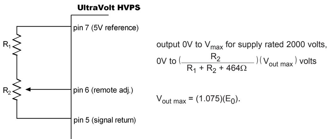
The sum ( $R_1 + R_2$ ) has to be much smaller than the input impedance of the *Remote Adjust Input* terminal (1M $\Omega$ ) and large enough not to load down the 5V reference supply. For example, ( $R_1 + R_2$ ) could be 50k $\Omega$  and satisfactory operation would result (with a maximum upper limit of 1.065 times the supply voltage rating).
