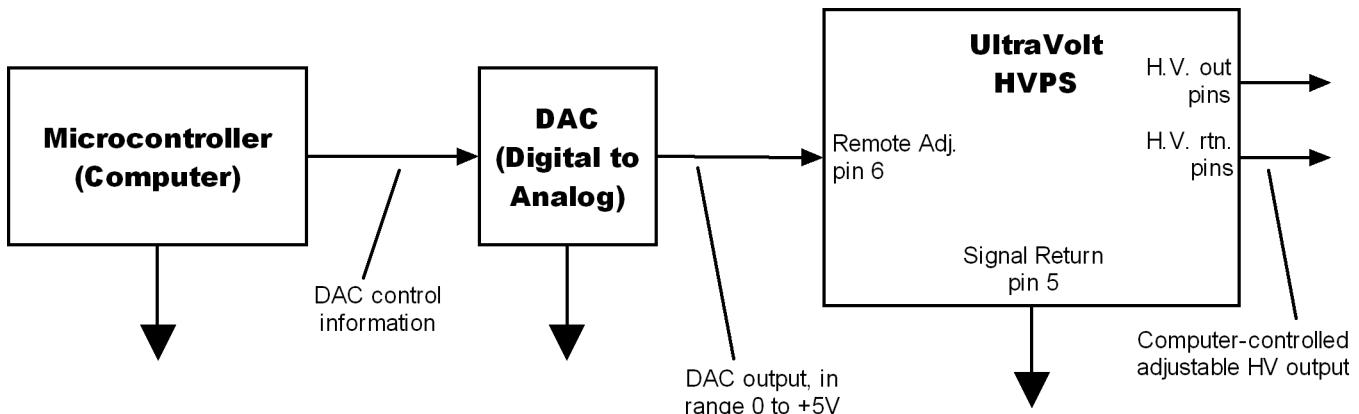
The UltraVolt high voltage power supply can also be programmed with a 0–10V DAC, Op Amp, or other control voltage using a resistive divider. For divider design purposes, the input impedance of the *Remote Adjust Input* terminal is  $1M\Omega$ . An example of a suitable divider for this application is as follows:
