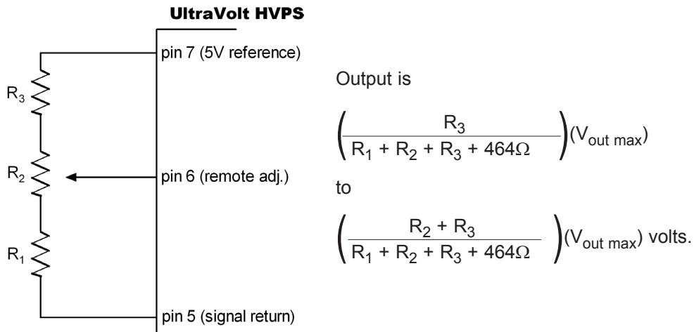
Although these examples deal with either positive or negative power supplies, the same circuits and theory can be used to analyze and to design positive and negative power-supply control systems. Each application noted here can be used with both negative or positive supplies with a slight modification to the formula: the variable  $V_{\text{pin6}}$  for positive supplies will be replaced by  $(5 - V_{\text{pin6}})$  to yield the output of the negative supplies.
