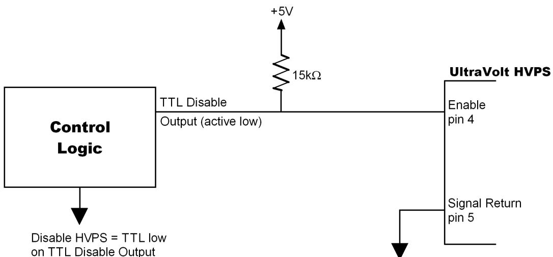
The  $15\text{k}\Omega$  resistor will ensure the *Enable/Disable* terminal stays at a voltage level that will force the HVPS to remain enabled until the TTL Disable Output signal goes low. When the TTL Disable Output goes low, the high-voltage power supply is forced into the disabled state. It should be noted, the HVPS has an internal,  $5.11\text{k}\Omega$  pull-up to +5VDC.
