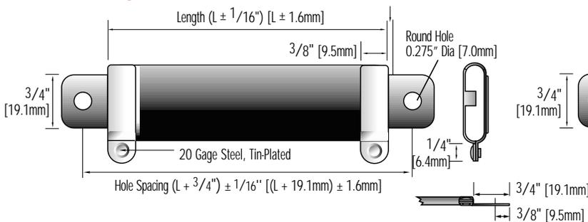
**Figure 6. With Standoff Axial Tabs (H2)**
