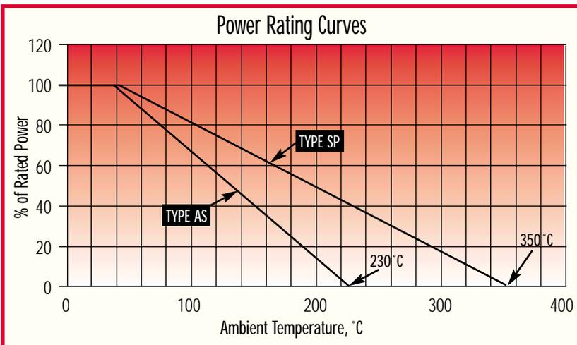
Power ratings are based on maximum allowable surface temperature in still air at 40°C ambient temperature.
