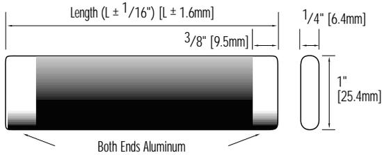
**Figure 2. With Straight Radial Tabs (G1)**
