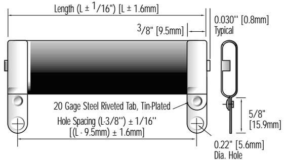
**Figure 3. With Right Angle Radial Tabs – same direction – (G2)**
