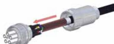
Screw housing adapter (6) to housing basis (7)
