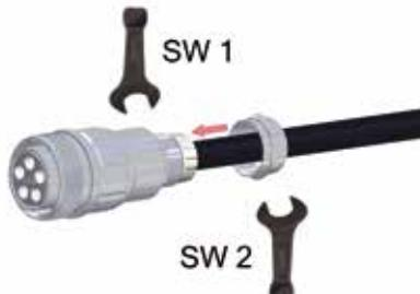
Screw cable gland cap to cable gland basis
