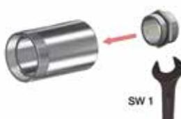
Screw cable gland basis (3) to housing adapter (4)
