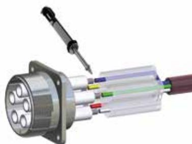
Solder one conductor on each female contact
