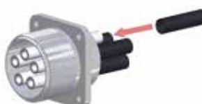
Put shrinking tubes (1) on insulation tubes on rear side of connector housing (3)
