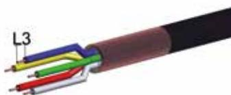
**Remove dielectric insulation of single wires
