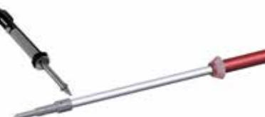
**Solder contact (8) on conductor**
