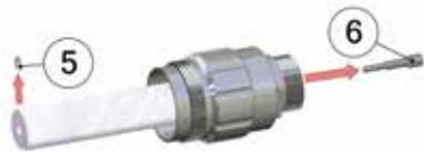
Remove snap ring (5), take out male contact (6) from insulation part (4)
