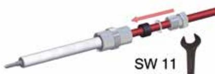
Completely slide clamping rubber (4) and washer (3) into basic part (6). Close housing with screw (2) (tightening torque = 3 Nm)
