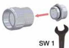
Screw cable gland basis (4) to housing adapter (5)
