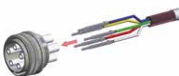
Slide contacts (7) completely into insulation tubes (5)
