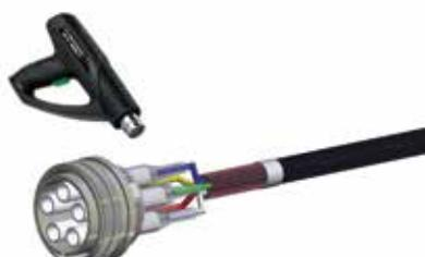
Place shrinking tubes on insulators. Tubes shall cover both insulators and wires. Then shrink tubes. Shrink temperature 100° C
