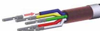
Crimp or solder female contacts (2) on conductor
