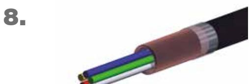
Remove any filling elements from cable
