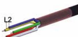
Remove dielectric insulation of single wires
