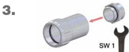
Screw cable gland basis (4) to housing adapter (5)
