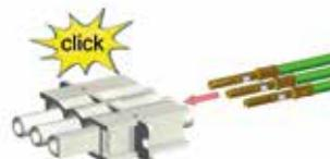
**Slide contact (2) completely into connector shell (3) until contact snaps**
