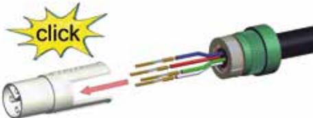
Slide contacts (5) completely into insulation part (6) until contacts snap
