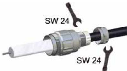
Screw cap (1) onto housing (3)
