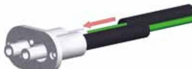
**Slide shrinking tube (1) on connector shell (3)****8.**
