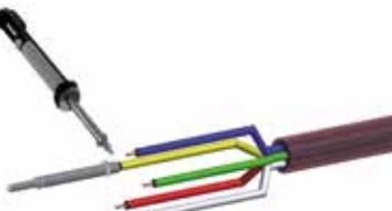
Solder one male contact (2) on each conductor
