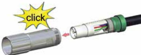
Slide insulation part (6) into housing (7) until insulation part snap in
