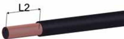
**Carefully remove cable jacket ( $L2 = \text{min. } 30\text{mm}$ )**
