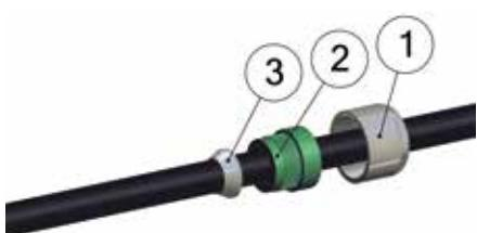
Place cap (1), clamping rubber (2) and outer cone (3) on cable
