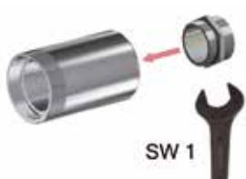
**Screw cable gland basis (3) to housing adapter (4)**
