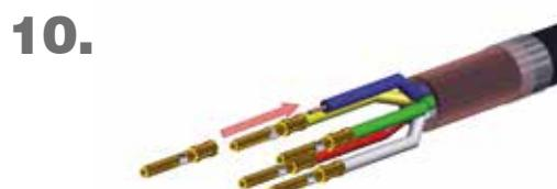
Crimp or solder female contacts (1) on conductor
