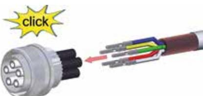
Slide female contacts completely into insulation tubes until contacts snap into place
