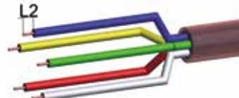
Remove dielectric insulation of single wires
