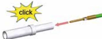
Slide contact (2) completely into connector shell (3) until contact snaps
