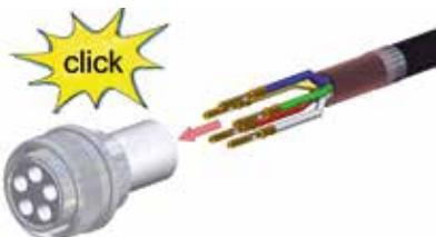
Slide female contacts (1) completely into housing basis (6) until contacts snap into place
