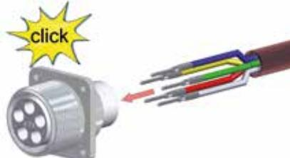
**Slide contacts (1) completely into connector shell (2) until contacts snap into place**
