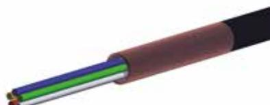
**Remove any filling elements from cable**
