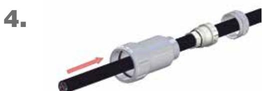
Place cap (2), sealing insert (3) and housing adapter (5) on cable.
