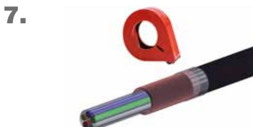
Fix shield braid with tape
