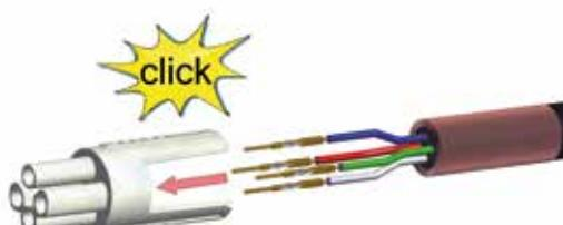
**Slide contacts (1) completely into insulation part (2) until contacts snap**
