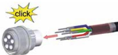
Slide contacts completely into housing basis until contacts snap into place
