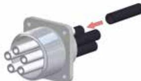
Put shrinking tubes on insulation tubes on back of connector housing.
