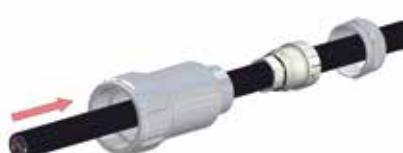
Place cap (3), sealing insert (4) and housing
