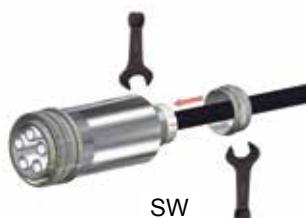
Screw cable gland cap (1) to cable gland basis (3)
