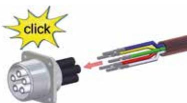
Slide contacts (2) completely into insulation tubes until contacts snap into place
