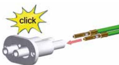
**Slide contact (2) completely into connector shell (3) until contact snaps**
