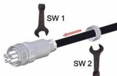
Screw cable gland cap (3) to cable gland basis (4)
