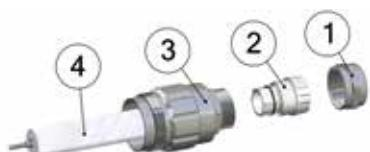
Remove cap (1) and take out sealing insert (2) from housing (3)
