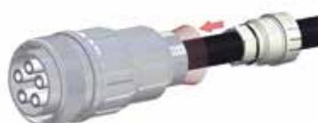
Completely slide seal insert under shield braid into cable gland basis
