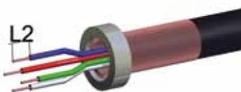
Remove dielectric insulation of single wires ( $L2 = 5\text{mm}$ )
