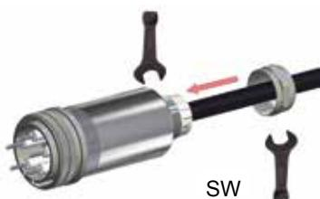
Screw cable gland cap (1) to cable gland basis (3)
