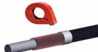
Fix shield braid with tape
