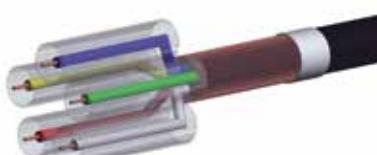
Place shrinking tubes on single wires.
