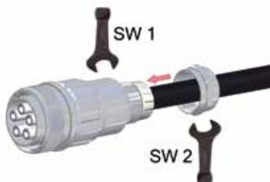
Screw cable gland cap to cable gland basis
