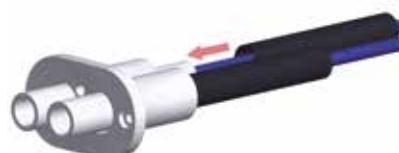
Slide shrinking tube (1) on connector shell (3)
