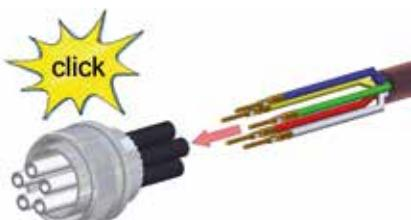
Slide male contacts (2) completely into insulation tubes until contacts snap into place
