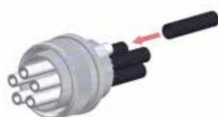
Slide shrinking tubes (1) on insulation tubes on rear side of housing basis (7)
