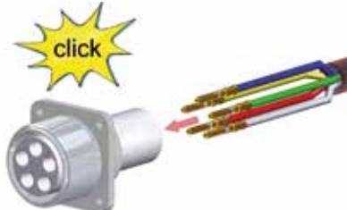
**Slide contacts completely into connector shell until contacts snap into place**
