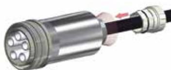
Completely slide seal insert (2) under shield braid into cable gland basis (3)
