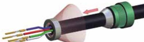
Completely widen shield braid. Push outer cone (3) and clamping rubber (2) under shield braid against inner cone (4) until shield braid clamps between outer cone (3) and inner cone (4)
