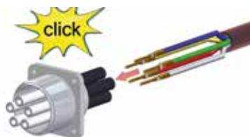
Slide contacts completely into insulation tubes until contacts snap into place
