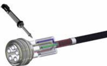
Solder one conductor each on a female contact
